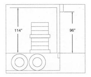
Figure 1 Eight foot (96") high doors can accommodate many loading operators when loading operations where height is not critical to product arrangement.
