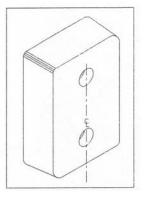
Figure 1 Fabric reinforced masticated rubber, shaped with lag bolt holes
