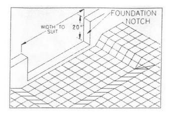
Figure 1 Pour in Place Installation (1)
