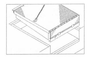
Figure 1 Sufficient Curb Angle must be provided for proper installation.
