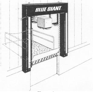
Figure 2 Three Sided Pit Installation
