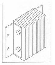
Figure 2 Fabric reinforced rubber pads, laminated and secured between steel angles
