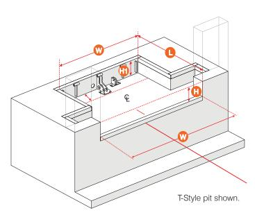
\*Concrete must be minimum 8" (203 mm) thick.
